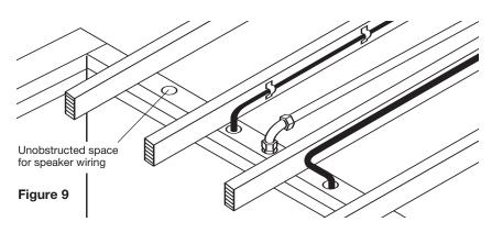
When you don't have access above or below the wall, try to estimate the existing wire and pipe locations from the positions of electrical outlets and plumbed fixtures on both sides of the wall. Take a look at the outside of your house too, sometimes conduit, vents or drain pipe will be visible that give useful information. Choose the route with the fewest potential obstacles.
